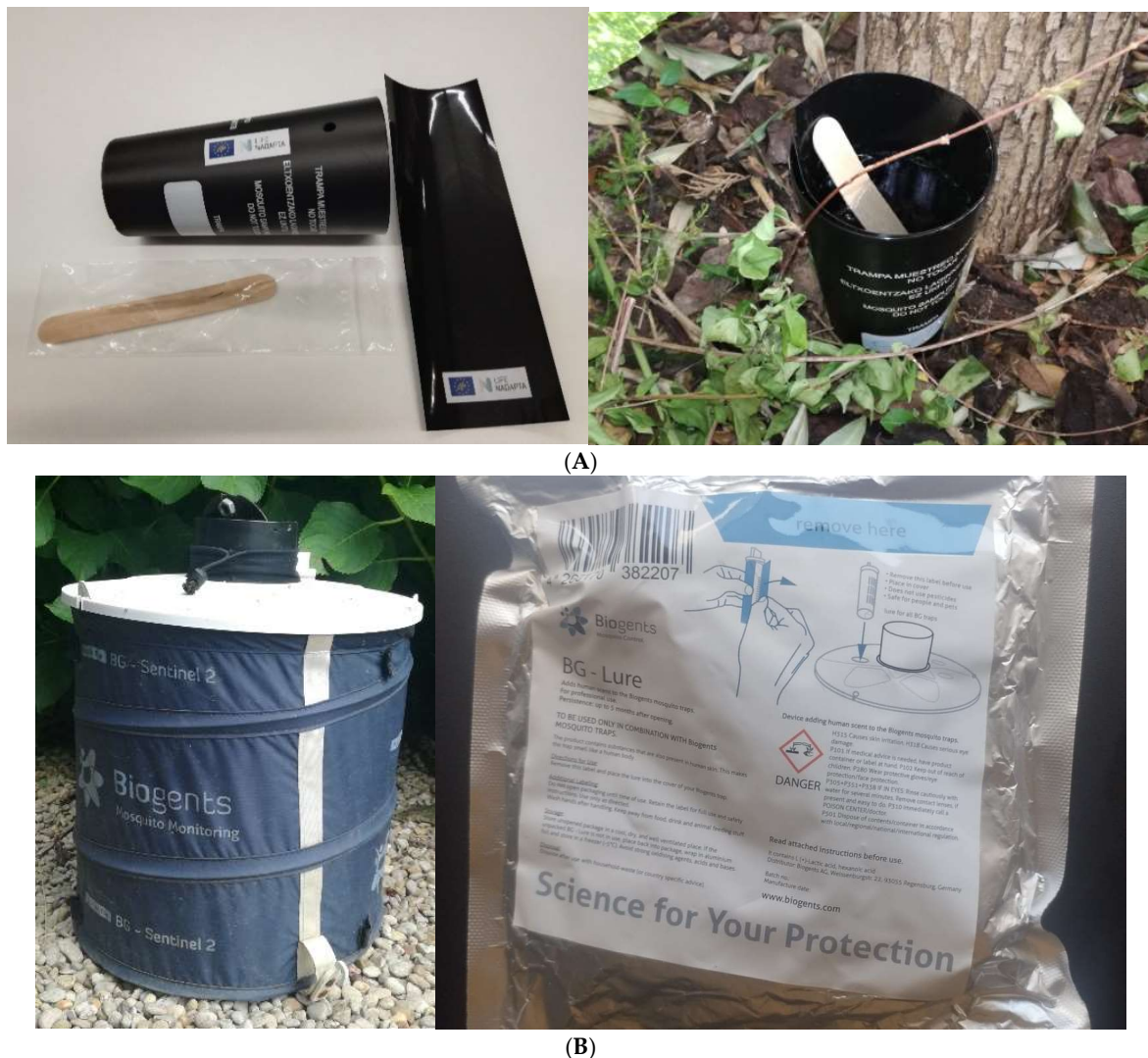
Figure 2. Traps employed. (A) One ovitrap dismantled and another already installed. (B) An adult trap and the BG-Lure product.
