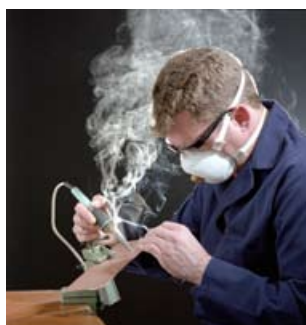
Figure 45 Soldering with and without Tyndall illumination
