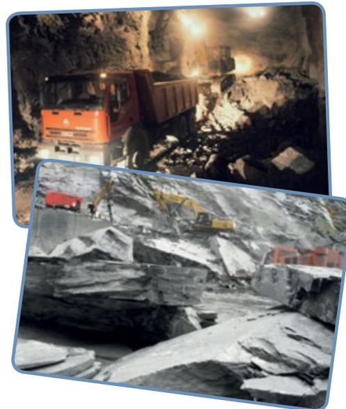
Other times, the minerals are in shallow deposits and are mined in open mine pits. The surface rock is broken with controlled blasts or by mechanical methods such as saws
